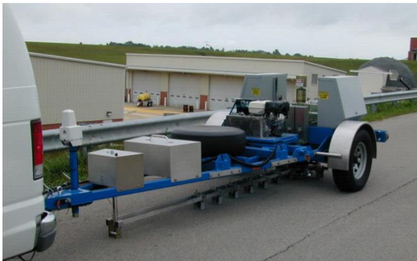
Figura 1: FWD modelo Dynatest® (FHWA, 2017)
